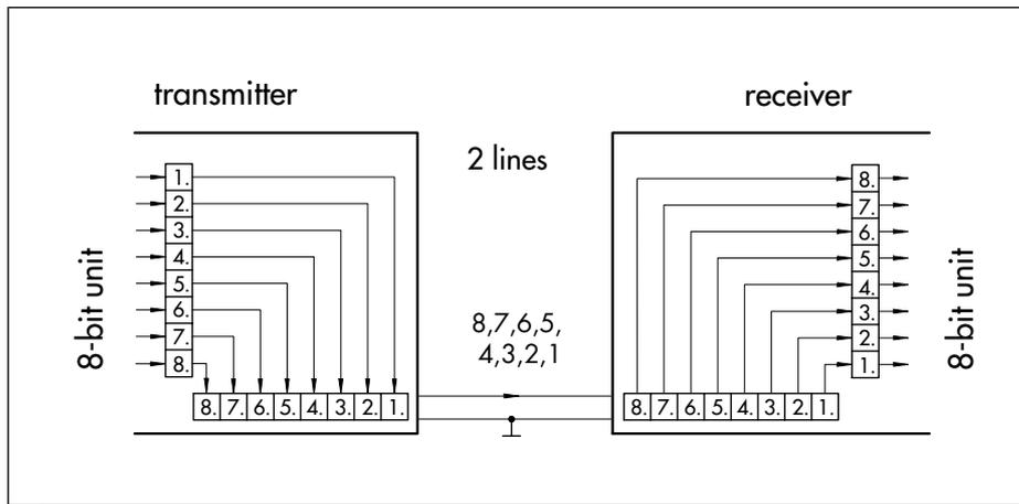
Fig. 9: Serial data transmission
