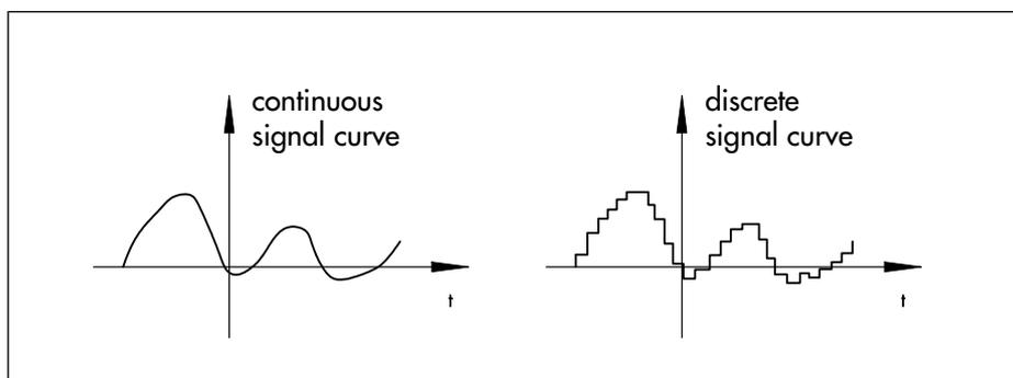
Fig. 1: Analog and discrete signal curves
