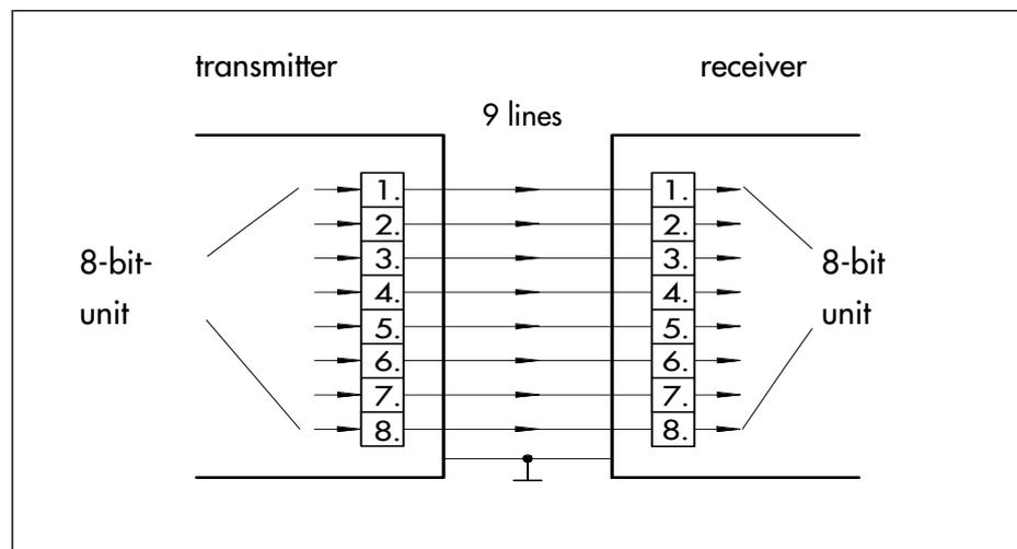
Fig. 8: Parallel data transmission
