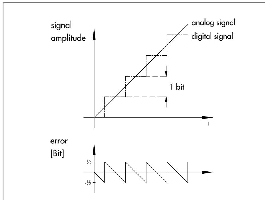
Fig. 3: Quantization error caused by reduced discretization and sampling rate
