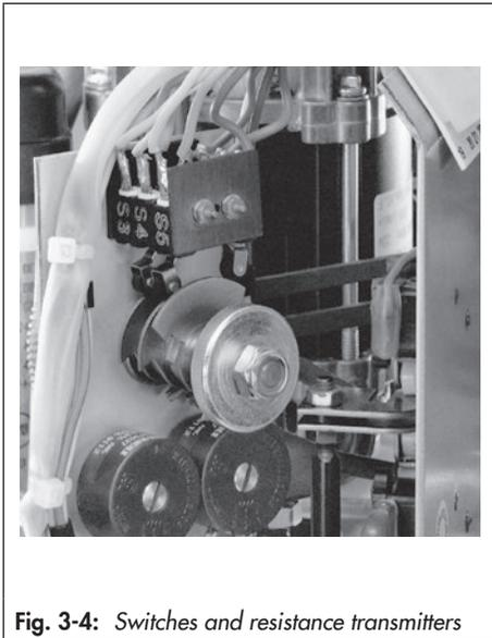
Fig. 3-4: Switches and resistance transmitters
