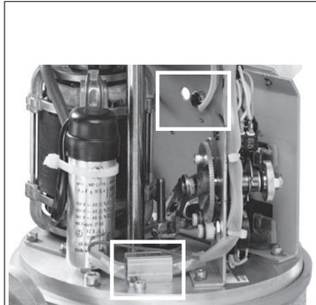
**Fig. 5-4:** Heating resistor (bottom), temperature switch (top)
