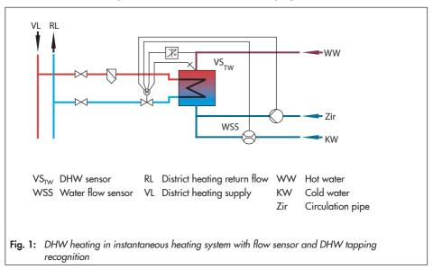
The DHW temperature is controlled to the set point temperature in DHW heating in instantaneous heating systems:
